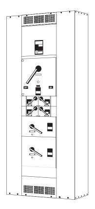
Siemens branch fusible switches are available with ampere ratings from 30 to 1200 amps.
