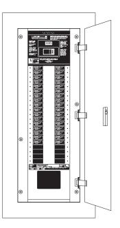
The following information gives various S2 rating ranges. Refer to Siemens Speedfax when ordering specific panelboards. The type of branch, main and subfeed breakers vary with the panelboard and application requirements. Only one subfeed breaker is allowed in the S2 panelboard, except 400 A and 600 A panelboards can have two QJ subfeed breakers.
