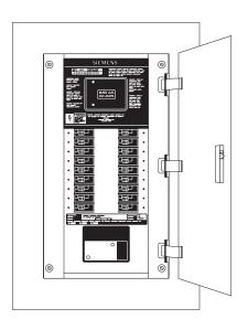
The following information gives various S1 rating ranges. Refer to the Speedfax catalog when ordering specific panelboards. The type of branch, main and subfeed breakers vary with the panelboard and application requirements. Only one subfeed breaker is allowed in the S1 panelboard, except 400 A and 600 A panelboards can have two QJ subfeed breakers.
