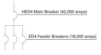
Series-rated breaker combinations must be tested in series in order to be UL listed. Siemens series-rated breakers are listed in the UL "Recognized Components Directory" (yellow books) Volume 1. Selected series-rated breakers are listed in the Speedfax catalog. Your Siemens sales engineer can provide more information on Siemens series-rated circuit breakers.
