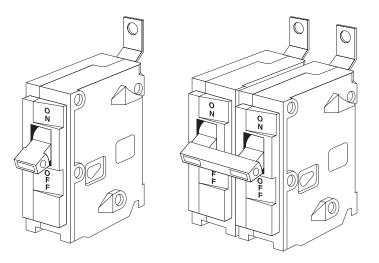
1-Pole Circuit Breaker One Overcurrent Device 2-Pole Circuit Breaker Two Overcurrent Devices
