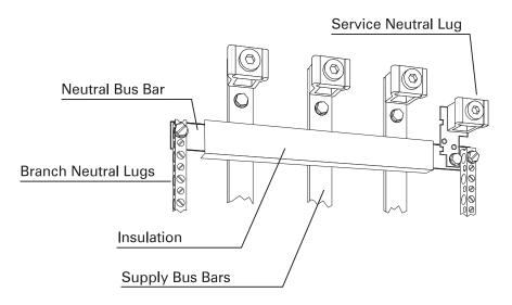
200% neutral Some loads can cause harmonics and non-linear loading on a distribution system. This requires special consideration when ordering a panelboard. One way to deal with non-linear loads is to double the capacity of the panelboard neutral. A 200% neutral can be factory installed or, in the case of the S1, S2 and SE, field installed.
