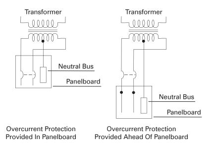
*NEC* makes an exception to this rule. A panelboard supplied by a single-phase transformer having a 2-wire (single-voltage) secondary can be protected by an overcurrent protection device located on the primary side of the transformer.
