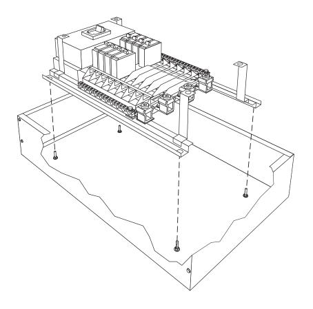
A <u>bus bar</u> is a conductor that serves as a common connection for two or more circuits. It is represented schematically by a straight line with a number of connections made to it. *NEC* article 384-3 states that bus bars *shall be located to be free from physical damage and shall be held firmly in place*. Standard bus bars on Siemens panelboards are made of aluminum, but copper bus bars are available as an option.
