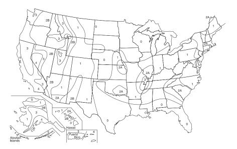
Siemens panelboards have undergone extensive seismic testing in order to obtain third party certification. Siemens panelboards will operate in zones 0, 1, 2A, and 2B with no modification. Panelboards that require zone 3 and 4 ratings are available with standard lead times.
