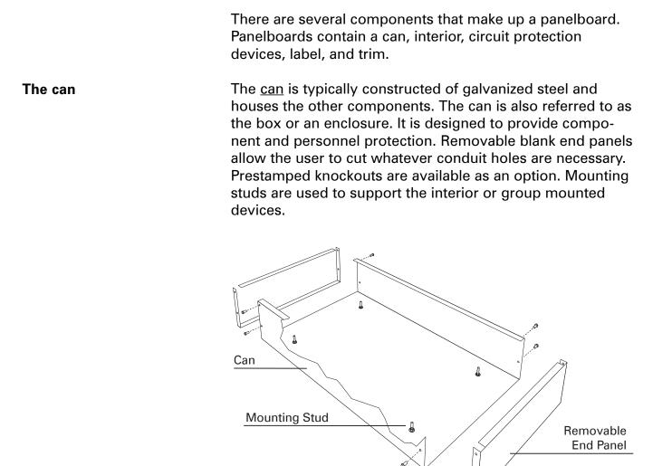
Siemens has a "Cans Ahead" program in which the can of some panelboards can be shipped separately of the interior and trim. This allows the contractor to install the can first before the wall is finished. For information on this program contact your Siemens sales representative.
