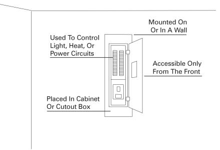
**Note:** Article 384 in the *National Electrical Code* covers panelboards. The basic requirements for panelboards are given in *NEC* Sections 384-13 through 384-16. You are encouraged to become familiar with this material.
