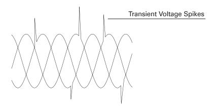
The most damaging voltage spikes are caused by lighting strikes. Although lightning strikes on high voltage lines are generally dissipated by utility transmission and arresters, a lighting strike on a power line several miles away still has the potential to cause extensive electrical damage. Damage to expensive electrical equipment can be either instantaneous or cumulative.
